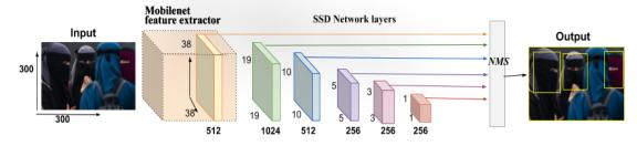
Figure 2. Mobilenet-SSD architecture composed of two parts: feature extraction and SDD
